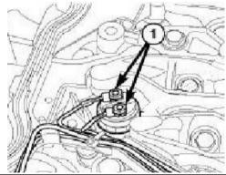
5. Remove the cylinder cover gasket.
