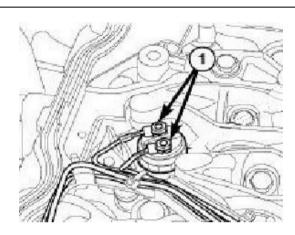
5. Reconnect both fuel injector harness connectors.
