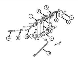
7.Remove the fuel injector connector nut.
