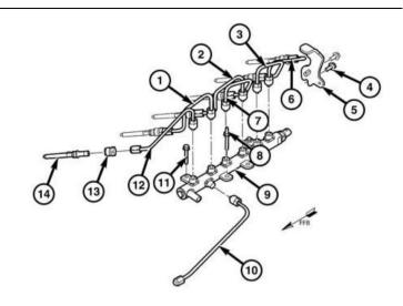
Connect the fuel injector solenoid wires and nuts to the top of the injectors. Tighten the connector nuts to 13 in-lb.
