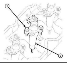
d. By hand, thread in the fuel injector connector tubes to ensure the fuel injector is centered and perpendicular to the connector tube. You can gently rotate the injector until the connector tube is correctly positioned. Do a preliminary tightening of the connector tube nut to 133 in-lb.
